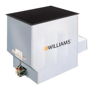
The combustion chamber is precision-formed, continuous-seam welded 18-gauge steel, and warranted for 10 years against rust out or burnout. The outer casing is constructed of heavy-duty galvanized steel, lapped and spot-welded for rugged durability.
