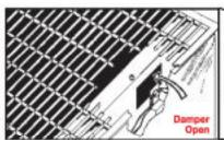
Setting No. 1 - In mild weather, operate furnace with damper open. Furnace will cycle on and off maintaining a moderate grill temperature and an even room temperature.
