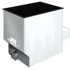
The combustion chamber is precision-formed, continuous-seam welded 18-gauge steel, and warranted for 10 years against rust out or burnout. The outer casing is constructed of heavy-duty galvanized steel, lapped and spot-welded for rugged durability.
